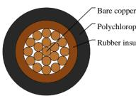
Bare copper conductor Polychloroprene rubber outer jacket Rubber insulation
